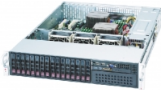
Figure 4 - A 16 hard drive, 2U, rack mount server
